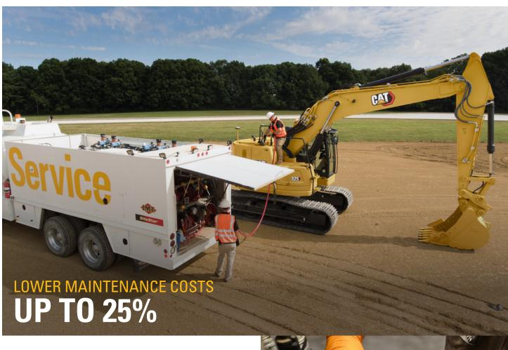
With extended and more synchronized maintenance intervals, you get more done at a lower cost compared to the 325F. Consolidated filter locations make service faster. Hydraulic, air, and fuel tank filters have increased capacity and longer life.
