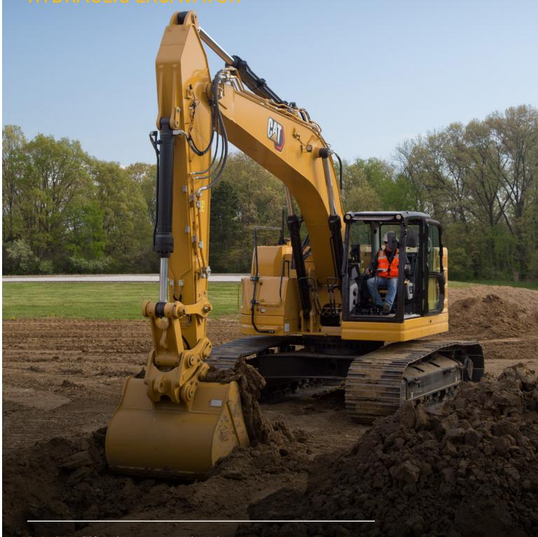
Engine Power (ISO 9249) Operating Weight 204 kW (273 hp) 34 900 kg (77,000 lb)—36 300 kg (80,000 lb)
