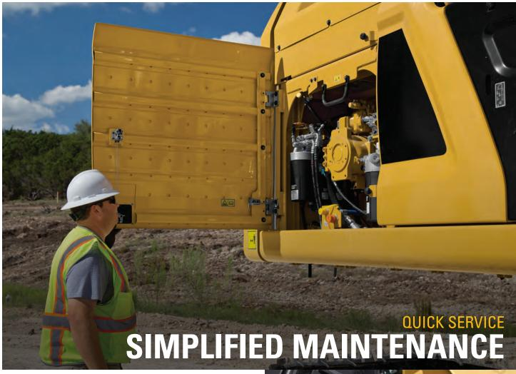
With extended maintenance intervals, you get more done at a lower cost. Consolidated filter locations make service faster. Hydraulic, air, and fuel tank filters have increased capacity and longer life.
