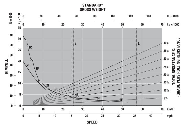
1C – 1st Gear (Converter Drive)
