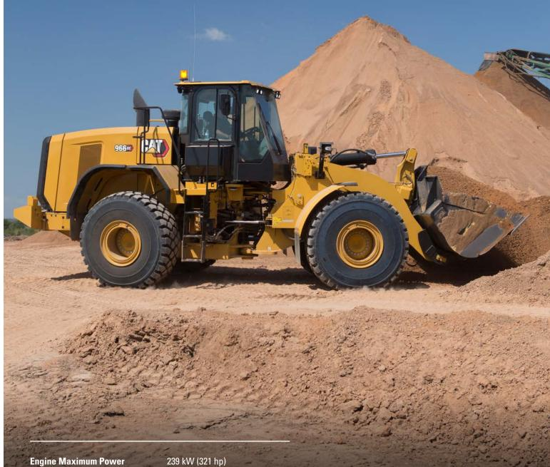
Engine Maximum Power Operating Weight Bucket Capacities 239 kW (321 hp) 21 781 kg (48,018 lb) 3.2-7.1 m³ (4.25-9.25 yd³)
