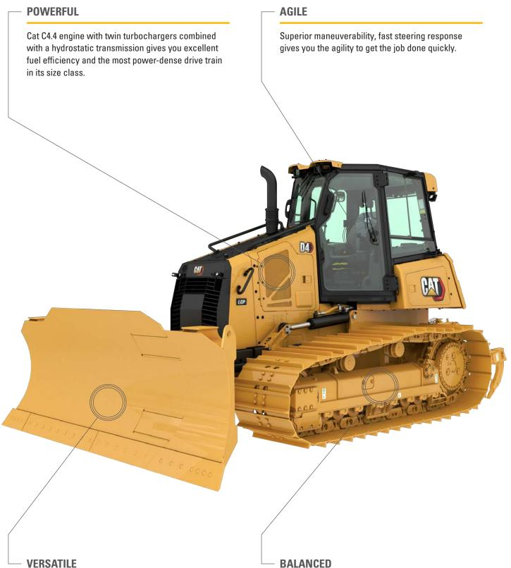
Variable Pitch Angle Tilt (VPAT) blade gives you the width and capacity to move material, as well as the finesse you need for smooth finish grades. Foldable VPAT option available for narrower transport width.
