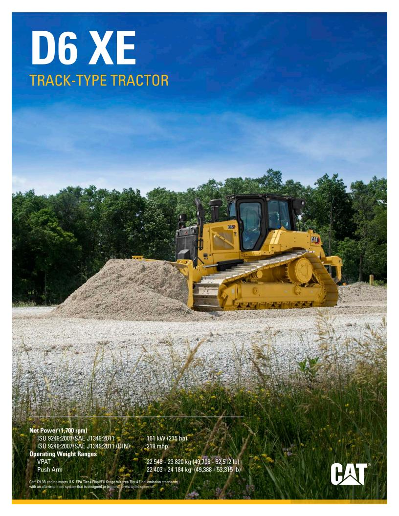
The Cat® D6 XE is the world's first high drive Electric Drive dozer, offering you the highest level of productivity, fuel efficiency and ease of operation. With next-generation Electric Drive technology there are no gears to shift, so you experience constant power to the ground, greater agility and faster cycle times.
