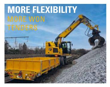
As an option, machine is equipped with pneumatic and electric features to allow towing of UIC-type wagons or rail trailers. Strong towing capacities allow up to 220 t with 8 wagon axles. Machine and wagon are easily and safely coupled using a certified tow bar and an automatic coupling system. New air pressure strategy allows saving time and keeps downtime to a minimum when convoy is brought to a stop. Time gain is about 60% when keeping pressure to 3 bar in tank.
