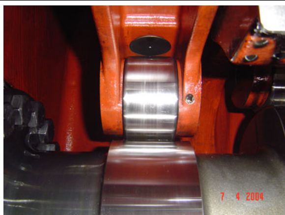
Inlet roller and cam after 70 operating hrs.
