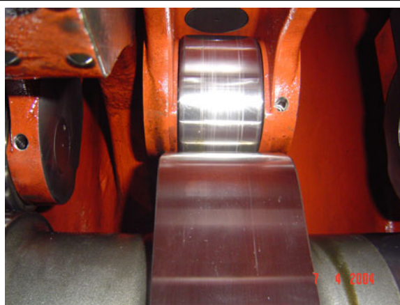
Exhaust roller and cam after 70 operating hrs.
