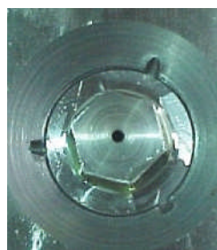
New production variant with hexagon head and locking. (Check carried out)
