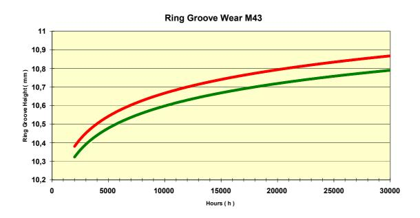
In the attached diagram considerably more than 90 % of the mean values measured at 4 points in the ring groove are below the lower green line. (measured 2mm from the outside, as shown on the standardized Measuring Sheet "Piston")
