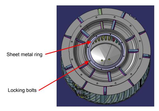
Investigations carried out in-house have shown that the design and quality of the bonding now being used for the filter silencers does not meet all the requirements necessary for reliable operation of the turbocharger. It has therefore been decided to lock the sheet metal ring in position by means of 8 bolts in addition to the bonding. These bolts are of a special design with an integrated verbus-ripp disc. Loctite will also be used to prevent loosening of the bolts.
