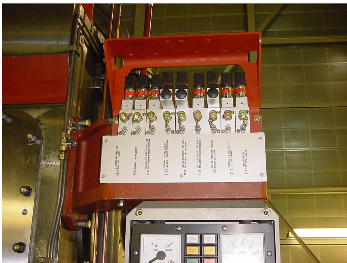
Identification plate with all engine measuring points
