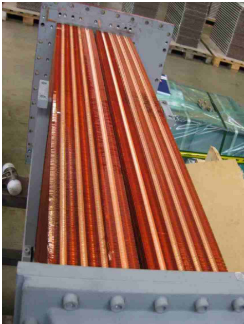
Missing row of tubes
