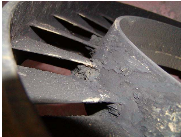
Examples of an excessively dirty nozzle ring
