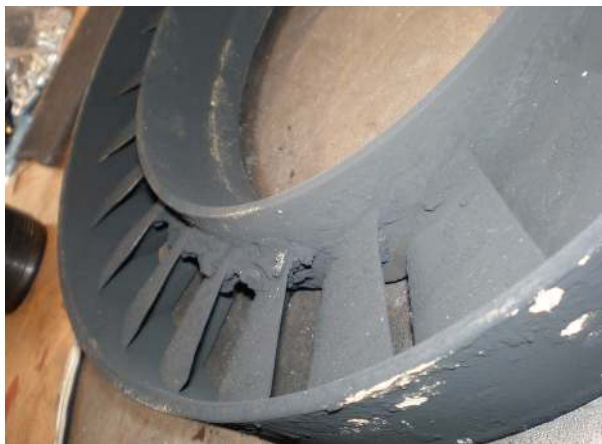
Examples of an excessively dirty nozzle ring
